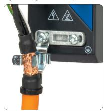
Kollmorgen Essentials Cables are supplied with the shield connection clamp. Push the cable into the spring clamp so that the exposed cable shield makes good contact with the shield clamp.
