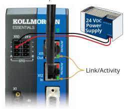
Confirm that the link LEDs on the drive (green LED on the RJ45 connector) and on your PC are both illuminated. If both LEDs are illuminated, then you have a working electrical connection.
